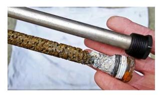
An anode rod is a sacrificial steel core wire wrapped with aluminum, magnesium, or zinc. Anode rods work by attracting corrosive particles found inside your water heater tank to protect the tank liner and reduce the risk of it bursting.
